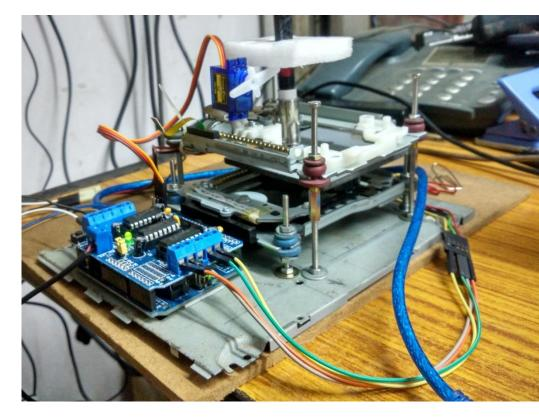
A weekend project on making a CNC plotter using junk CD drives. The stepper motor and lead screw mechanisms were salvaged from old CD drives. Using an additional servo motor a fully functional mini CNC plotter was built. Open source code from arduino, processing and inkscape was used to read data from the computer and scribe it using the plotter.
