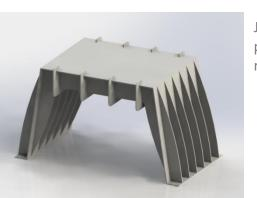
Joined by notches and no permanent joints allows for easy replacement of components
