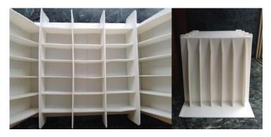
Internal rib structure allows to support load upto 3 kg.
